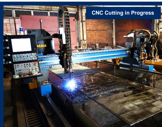
Plasma Cut M/S Plate 16mm thk
