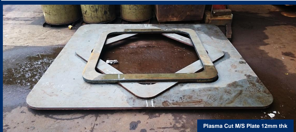
Plasma Cut M/S Plate 12mm thk
