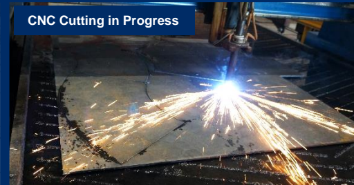
Plasma Cut M/S Plate 16mm thk
